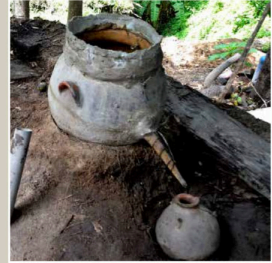
Filipino-style clay pot stills with a copper condenser
