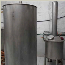
Stainless steel still with a copper coil
