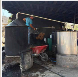
Stainless steel and copper coil alembic
